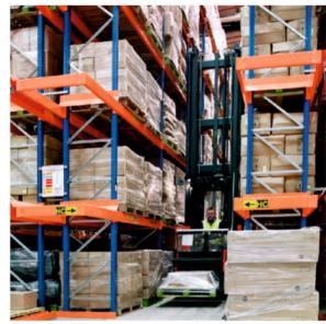
Radio Shuttle Pallet Racking
